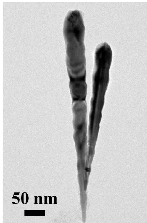
Figure 3. TEM micrograph showing two Pd nanothorns.
